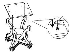
Remark: The bolts are pre-attached to bottom panel.
