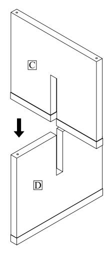
Assemble the two Legs into the X shape like the description above.
