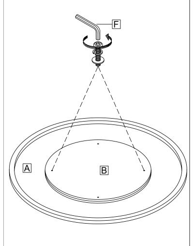
Remove Connecting Plate from the Table Top.
