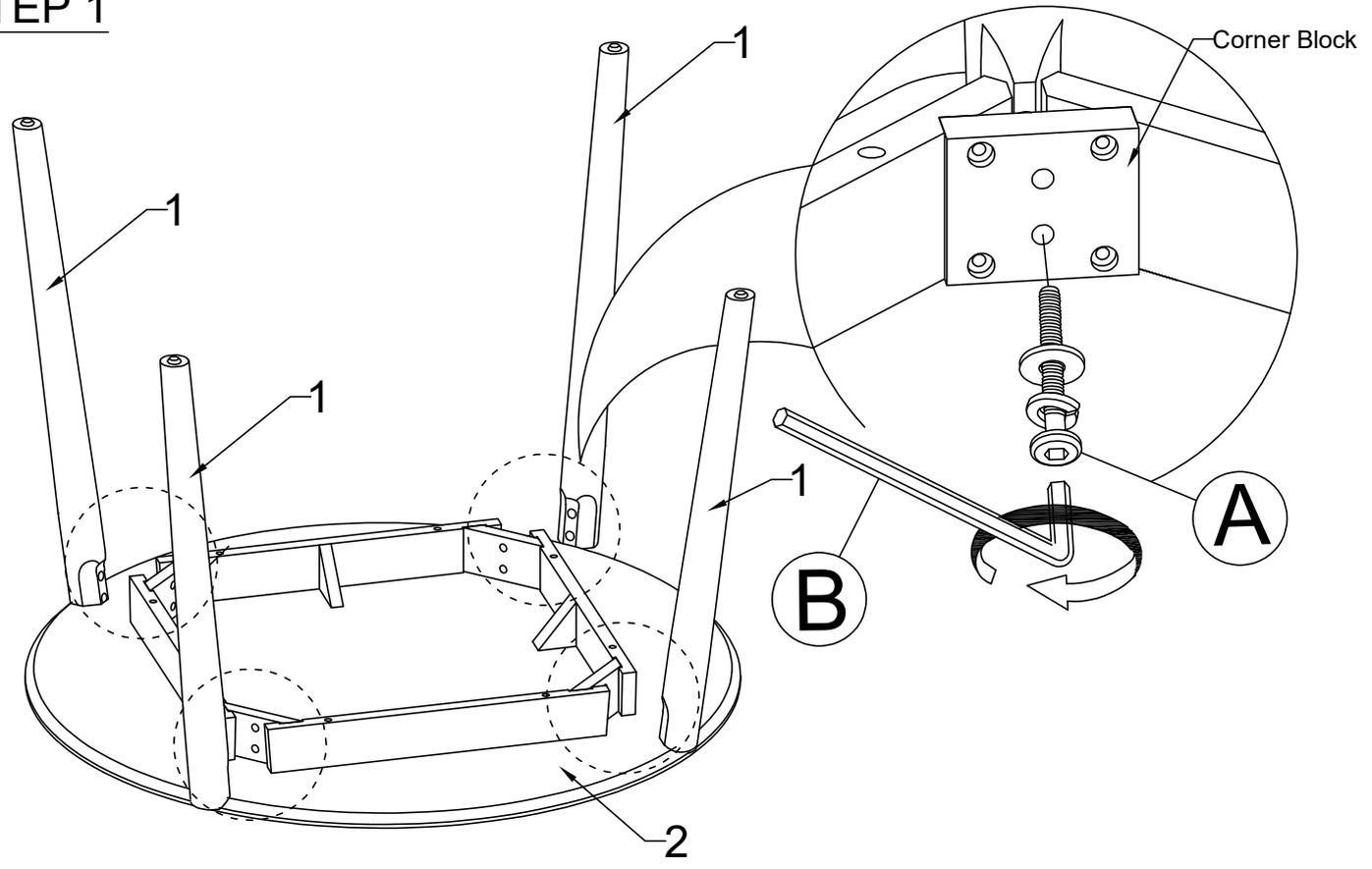
Place the table top on a smooth surface, insert JCBB Bolt (A) through the corner block of table top to fasten table leg (1). Use Allen Key (B) to tighten (A).
