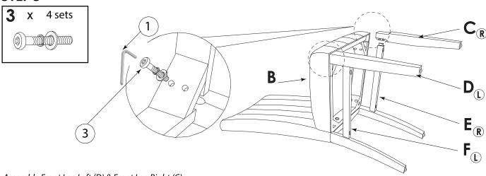
Assemble Front Leg Left (D) & Front Leg Right (C) by aligning Bolts (3) fitted with Spring Washer & Flat Washer.
