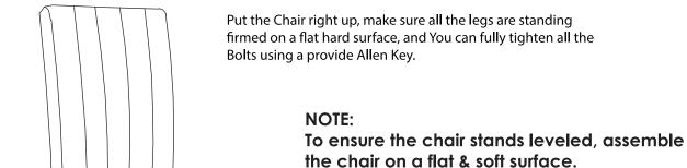
DO NOT tighten all bolts and screws until the chair is adjusted & balanced all the legs so that they do not wobble. Once adjusted, then fully tighten all the bolts and screws while making sure that the unit remains level on a flat surface.
