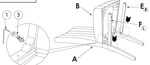
Insert Right Stretcher (F) and Left Stretcher (E) into the designated hole on Back Leg Frame (A)
