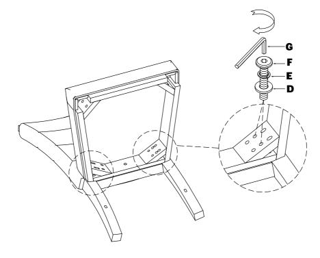
Step 3: Do not fully tighten the bolts
