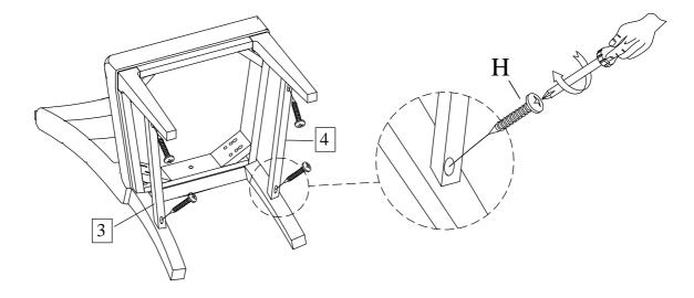
Step 5: Using the Allen key and a Phillips head screw driver, tighten all bolts.
