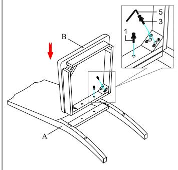
This step needs installation of two Bolts (#1) and four Bolts (#3).
