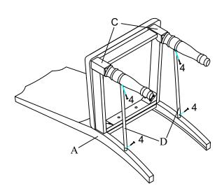
This step needs installation of four Screws (#4).
