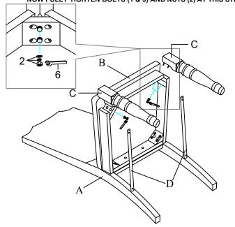
This step needs installation of four Nuts (#2).
