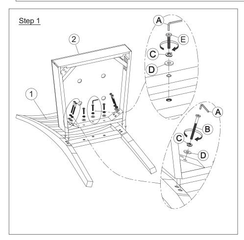
Lay flat the Backrest Assembly (1) to clean surface. Secure the Seat (2) with Allen bolt (B), Allen bolt (E), Lock washer (C) and Flat washer (D) using Allen key (A). Fully tighten all bolts.
