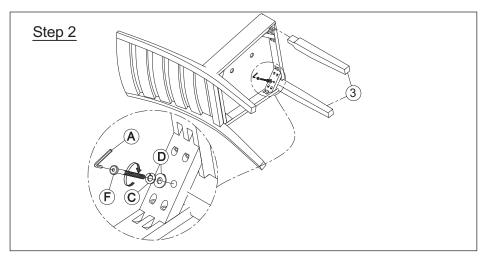
Attach the Front Legs (3) with Allen bolt (F), Lock washer (C) and Flat washer (D) using Allen key (A). Fully tighten all bolts.
