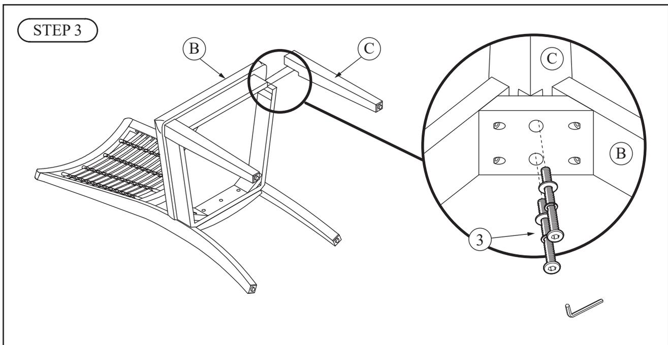
Attach Legs (C) to Seat (B) using 2 Allen Bolts, 2 Spring Washers, and 2 Flat Washers per leg. Tighten bolts using Allen Wrench provided. The assembly is now complete.
