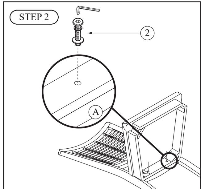
Secure Seat (B) to Back (A) using 3 Allen Bolts, 3 Spring Washers, and 3 Flat Washers.
