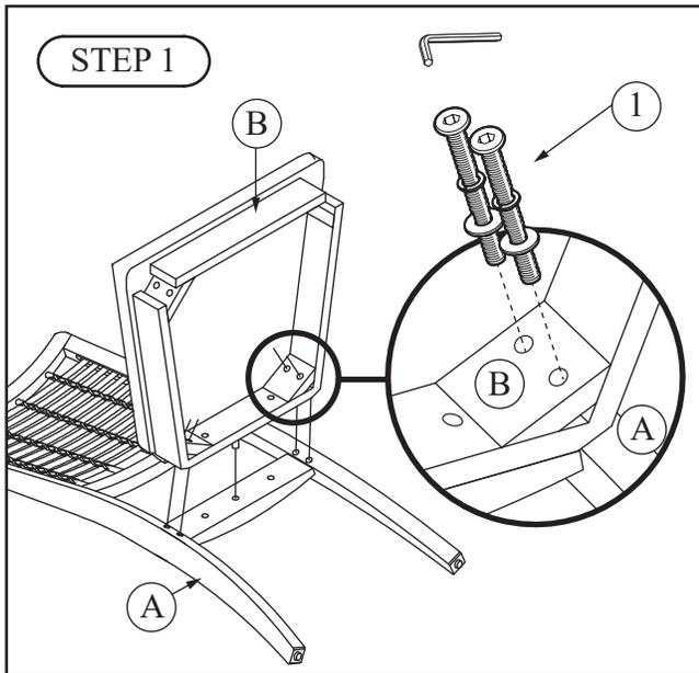
Begin assembly by attaching Seat (B) to Back (A) using 2 Allen Bolts, 2 Spring Washers, and 2 Flat Washers per side.
