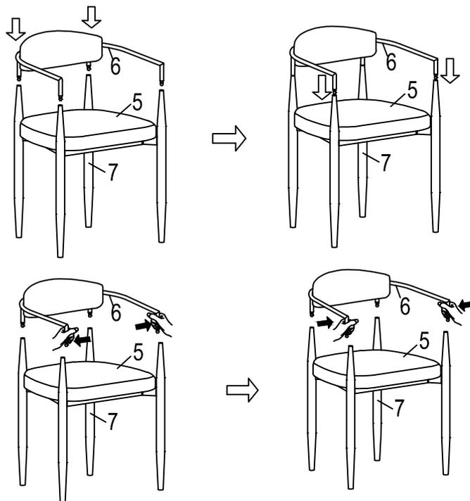
**Noted: If the metal on both sides of the armrest of the Backrest 6 is not aligned with the holes on the Metal frame 7, please gently use your hand to force them**
