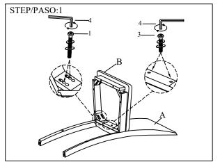
Assemble the seat frame corner with the chair back. Do not tighten all bolts until seat frame is fully assembly.
