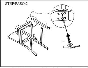
Assemble the front leg with the chair seat. Meanwhlie, put the side stretcher in correct position like picture showed.
