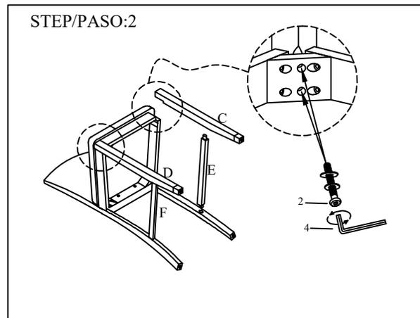
Assemble the front leg with the chair seat. Meanwhile, put the side stretcher in correct position like picture showed.
