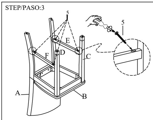
Assemble the side stretcher and front stretcher with the chair leg, Do not tighten all bolts until they are fully assembly.
