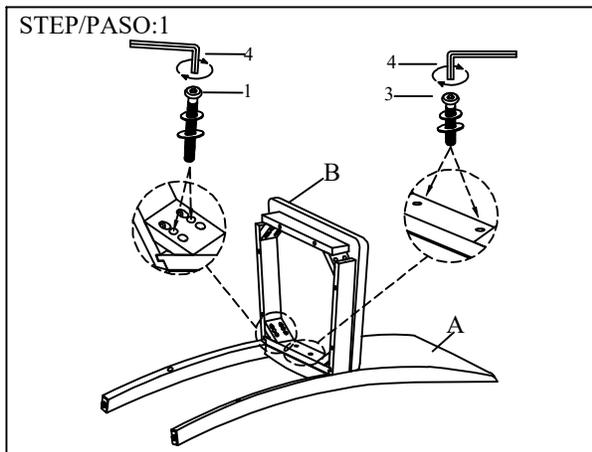
Assemble the seat frame corner with the chair back. Do not tighten all bolts until seat frame is fully assembly.
