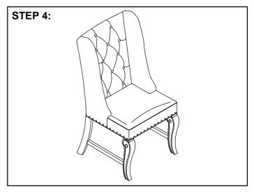
Turn host chair to the upright position, apply firm pressure to align and fully tighten all bolts and screws.
