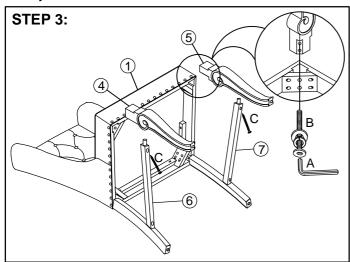
Attach the front legs to side stretcher and seat. Secure the side stretchers to the front legs.
