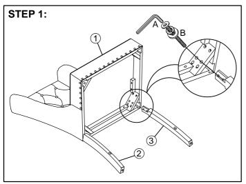
Attach the back legs to the seat frame with back Note: Do not tighten all screws & bolts until the seat is fully assembled.
