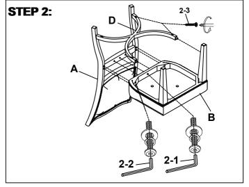
Attach the seat frame to the chair back and X stretcher to the chair back and front legs.
