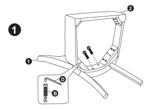
Insert the screws in the holes, then tighten, to 90%.
