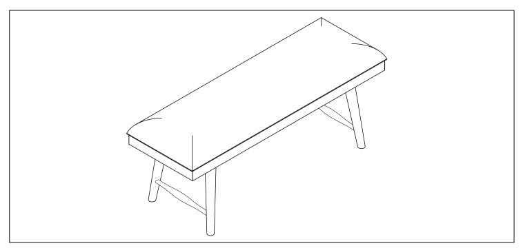
Stand bench up on an even surface and check that it is balanced. If there is a slight wobble, apply downward pressure in the corner where a leg is uneven. Keeping pressure in that corner, tighten all belts. If balanced, apply downward pressure evenly in the center and tighten all bolts.
