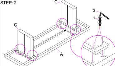
Place the bench top upside down. Attach the Bench Legs and Connecting boards to the table top.By inserting Bolt/ Lock Washer/ Flat Washer (1) and tighten with Allen Key (2).
