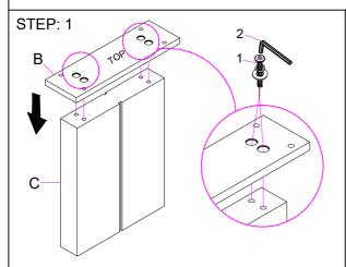
Attach the Connecting boards (B) to the Legs by inserting Bolt/ Lock Washer/ Flat Washer (1) and tighten with Allen Key (2).
