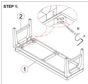
Do not tighten all the bolts until the assembly is completed.
