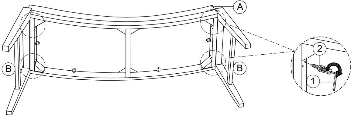
Attach Side Leg to Cushion Seat With Frame, with JCBC Bolt and Washers using Allen Wrench.
