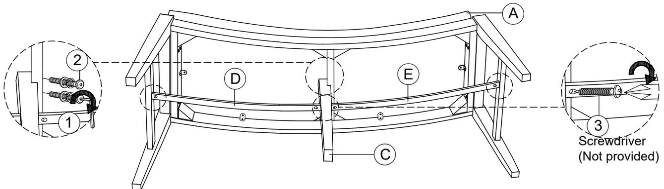
Attach Center Leg to Cushion Seat With Frame, with JCBC Bolt and Washers.
