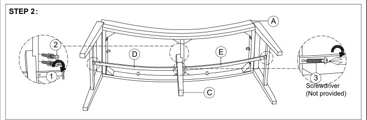
Attach Center Leg to Cushion Seat With Frame, with JCBC Bolt and Washers. Attach Left and Right Stretchers to Side Leg and Center Leg, then use Chipwood Screws to lock the Stretchers in place. Finally, tighten all JCBC Bolts using Allen Wrench.
