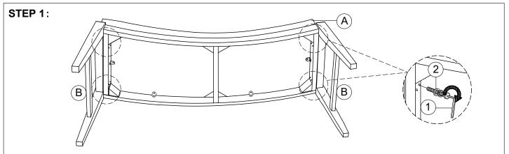
Attach Side Leg to Cushion Seat With Frame, with JCBC Bolt and Washers using Allen Wrench.
