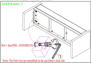
Assemble seat frame with the stretcher and side frame
