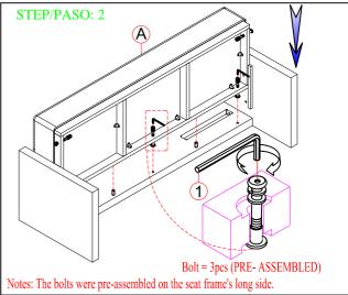
Assemble side frame with the stretcher
