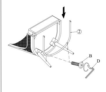
STEP 3: Attach Metal Stretcher (2) to Front legs (5), (6) by using Screw (C) with Screwdriver. And attach Front legs (5), (6) to Chair seat (1) by using Bolt (A) with Allen key (D).
