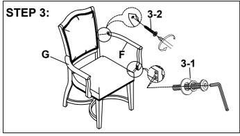
Attach the arms to the chair back and seat feame. Note: Do not tighten all screws & bolts until the seat is fully assembled.
