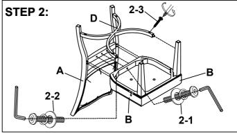
Attach the seat frame to the chair back and X stretcher to the chair back and front legs.
