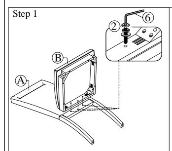
Attach the Seat Frame w/Seat Cushion (B) to the chair backrest of the Chair Back (A) by inserting Short Bolt/ Lock Washer/ Flat Washer (2) and tighten with Allen Key (6). Note: Do not tighten bolts until the seat is fully assembled.
