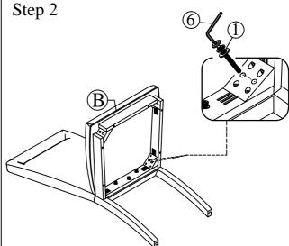
Insert Long Bolt/ Lock Washer/ Flat Washer (1) at the corner to the rear back legs of the Chair Back (A) and tighten with Allen Key (6).
