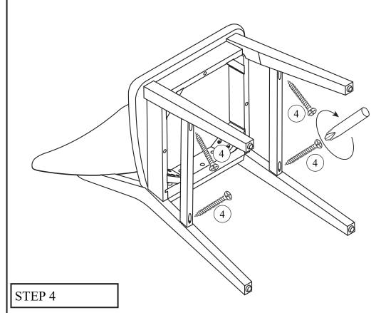
Turn up the chair, place it on level ground. Make sure the chair are not wobbling before fully-tighten all bolts in step 1 & step 2.
