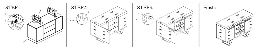
Lay the buffet upside down, on a carpeted or protective surface, to avoid damage. Attach the legs, using the provided screws and washers, aligning the holes, into the threaded inserts, tighten securely. Stand the buffet upright. The handles are mounted at the back of doors and drawers. Unscrew the handles from the back of doors and drawers. Put the handles on door/drawer fronts, use the same screws unfastened and then fasten the handles on the door / drawer fronts respectively
