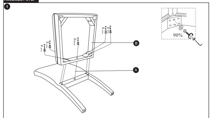
Put the Chair Back(A) on a non-abrasive table. Attach the Seat(B) to Chair Back(A) using five Bolts(D1,D3), five Spring Washers(E) and five Flat Washers(F) with the provided Allen Key(G). Do not fully tighten any bolt, but 90%.
