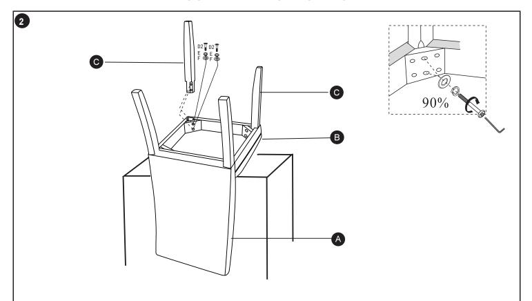
Put the Seat(B) on a non-abrasive table. Assemble Front Legs(C) to the front of the Seat(B) using four Bolts(D2), four Spring Washers(E) and four Flat Washers(F) with the provided Allen Key(G). Do not fully tighten any bolt, but 90%.
