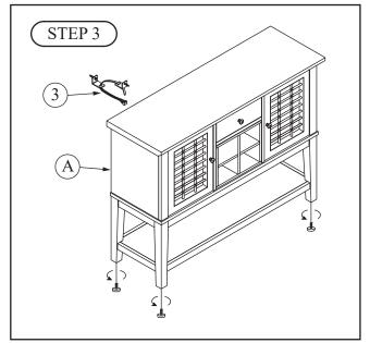
Tighten all bolts with Allen Wrench provided. Tighten levelers on bottom of legs. Attach Tip Restraint Kit (3) to back of Cabinet (A). The assembly is now complete.
