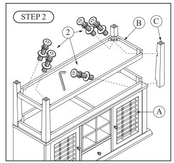
Attach Bottom Panel (B) to Legs (C) using 1 Allen Bolt, 1 Spring Washer, and 1 Flat Washer (2) per leg. Attach remaining Leg (C) using 2 Allen Bolts, 2 Spring Washers, and 2 Flat Washers (2) to the Cabinet (A) and 1 Allen Bolt, 1 Spring Washer, and 1 Flat Washer (2) to the Bottom Panel (B).
