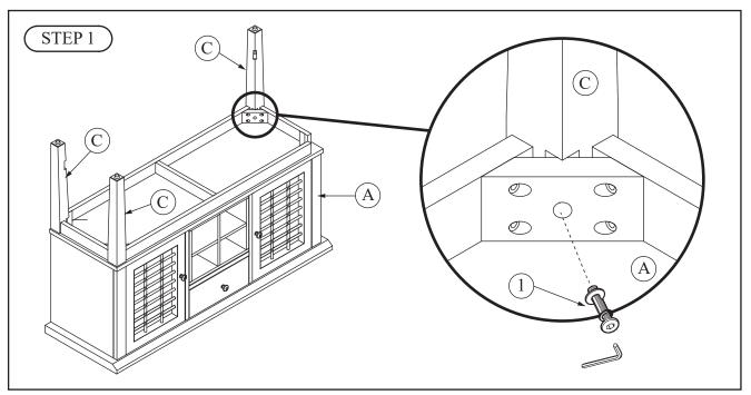
Attach Three of the Legs (C) to Cabinet (A) using 2 Allen Bolts, 2 Spring Washers, and 2 Flat Washers (1) per leg.
