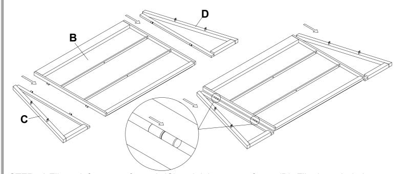
STEP: 2 Flip up left support frame L (C) and right support frame (D) .Flip down 2 shelves.
