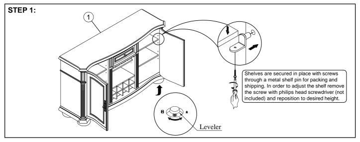
Turn server to the upright position. Apply firm pressure to align Leveler.
