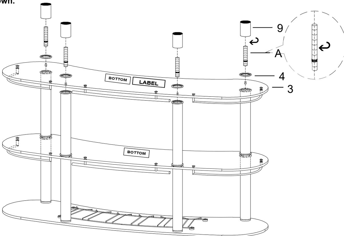
**Step 5) ATTENTION ! Re-checking all glass holder bolts (D) firmly and re-swivel all posts (8) & (9) bottom-up to make all firmly enough as below shown. Turn the bar table upside down by 2 strong persons carefully.**
