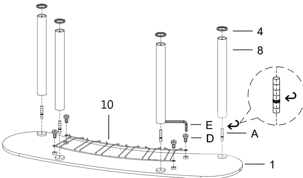
**Step 3) Put pre-assembled middle glass shelf (#2) on the frame then repeat to attach bolt (A), long post (#8) and plastic ring (#4) to pre-assembled middle glass shelf (#2) one by one bottom-up accordingly again.**
