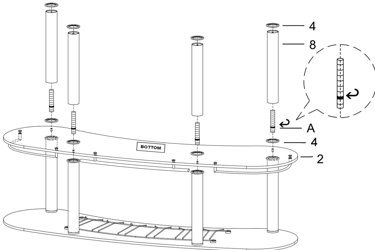
**Step 4) Put pre-assembled bottom glass shelf (#3) on the frame again then attach plastic ring (#4), bolt (A) and short post (#9) to pre-assembled bottom glass shelf (#3) as below shown.**
