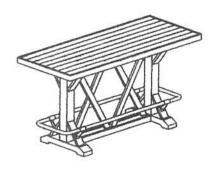
ADJUST ALL PARTS OF METAL FOOTREST IN PLACE AND FULLY TIGHTEN ALL BOLTS!
