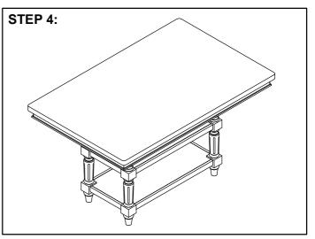
Turn the table upright. Apply firm pressure to align and fully tighten all bolts.
