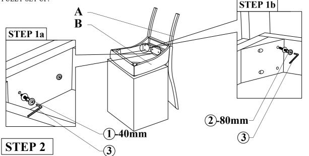
**Assemble FRONT LEG to SEAT as illustration shown.** DO NOT TIGHTEN THE SCREWS UNTIL FULLY SET UP.
