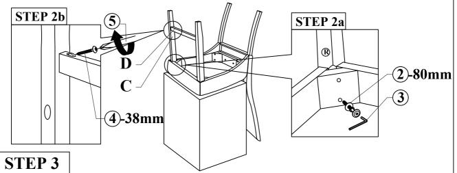
Assemble STRETCHER to LEG as illustration shown. (NOTE : USE HARDWARE IN BOX 4) TIGHTEN ALL THE SCREWS !!!
