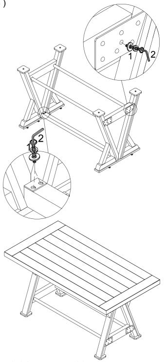
NOTE:DO NOT FULL TIGHTEN BOLTS UNTIL PARTS COMPLETE ASSEMBLED Cleaning instructions:Clean using soft cloth Made in Viet Nam
