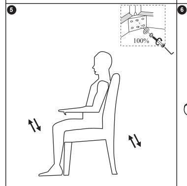
Seat on the chair, and wiggle. Ensure the chair is lever on the floor, then fully tighten all Bolts(1) with the provided Allen Key(5). Place the vinyl flap to the bottom of the Seat(B) using chair is completely assembled, and it is ready to use. the adhesive strips.
