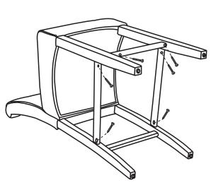
Put six Flat Head Screws (2) into the holes of Front Stretcher (D) and Side Stretchers(E), and fully tighten them. Now the
