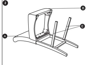
Inset the **CHAMFERRED END** of Side Stretchers(E) into the holes of Chair Back legs(B) as shown. Please don't assemble Side Stretchers(E) with any bolt or screw.
