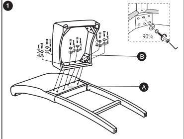
Put the Chair Back(A) on a non-abrasive table. Attach the Seat (B) to Chair Back(A) using six Bolts(1), six Spring Washers(3) and six Flat Washers(4) with the provided Allen Key(5). Do not fully tighten any bolt, but 90%.
