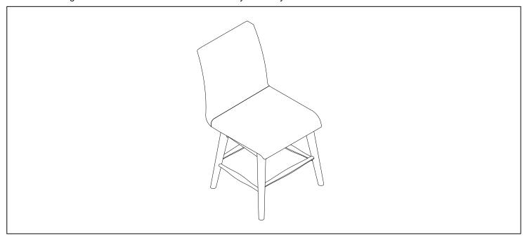
Stand chair up on an even surface and check that it is balanced. If there is a slight wobble, apply downward pressure in the corner where a leg is uneven. Keeping pressure in that corner, tighten all belts. If balanced, apply downward pressure evenly in the center and tighten all bolts.
