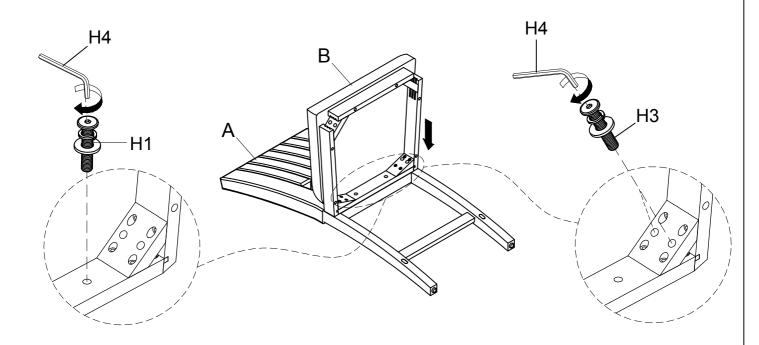
Attach the Seat frame to the chair backrest. Do not tighten all screws & bolts until the seat is fully assembly.
