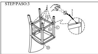
Assemble the side stretcher and front stretcher with the chair leg, Do not tighten all bolts until they are fully assembly.
