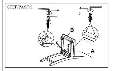
Assemble the seat frame corner with the chair back. Do not tighten all bolts until seat frame is fully assembly.
