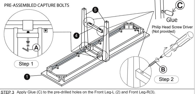
Place the Front Leg-L (2), Stretcher (4) and Front Leg-R(3) to corner of apron, then tighten the Flat Washer, Spring Washer and Bolt using the Allen Key (A) provided. Insert Screw(B) into Stretcher(4) through the pre-drilled holes, tighten it by using Philip Head Screw Driver (Not provided).
