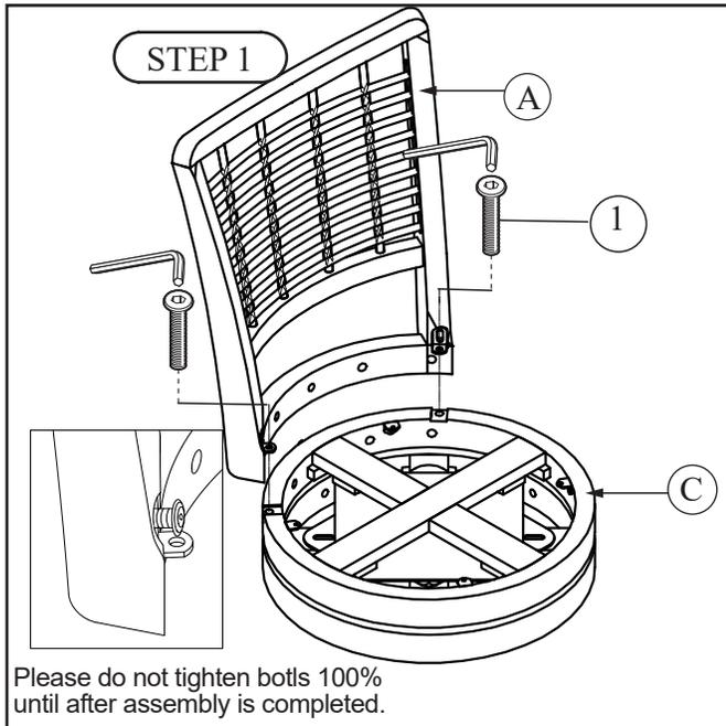
Please do not tighten bolts 100% until after assembly is completed.
