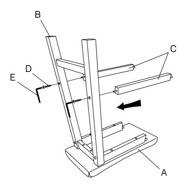
Line up of second Leg Frame (B) with screw holes on bottom of Seat (A) and attach with JCBC/W (D) using Allen Key (E). Do not tighten these screw all the way until you insert the Stretcher (C) when all holes are aligned. Tighten all remaining screw.
