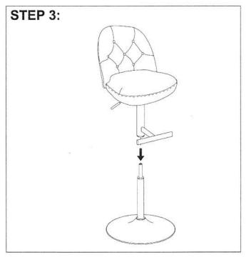
Turn assembled seat upright and slide the pole with footrest over the gas lift. Push down firmly until
