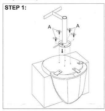
Attach the pole with footrest to seat ensuring the footrest points towards the front of the unit. Note: Do not over tighten the bolts.
