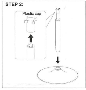
Insert the thick end of the gas lift into the base. Remove the top plastic cap for the following step.
