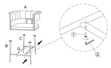
Attached the 2 stretcher to the leg rail with the M6 x 15 bolt.
