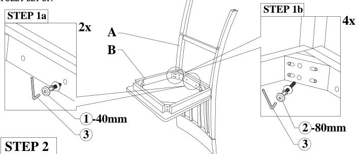
Assemble FRONT LEG to SEAT as illustration shown. DO NOT TIGHTEN THE SCREWS UNTIL FULLY SET UP.
