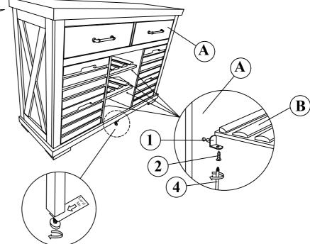
Adjust the level to make sure it touch the floor
