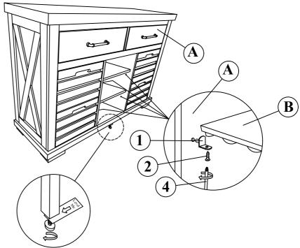
Adjust the level to make sure it touch the floor
