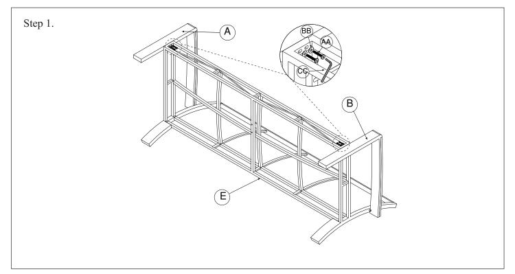
Assemble the side frame (A & B) into the seat frame (E) by bolt, flat washer. Using allen key to tighten all bolts
