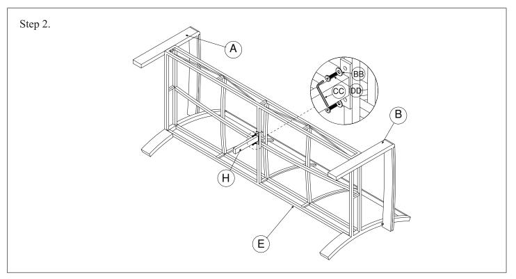
Assemble the leg (H) into the seat frame (E) by bolt, flat washer. Using allen key to tighten all bolts
