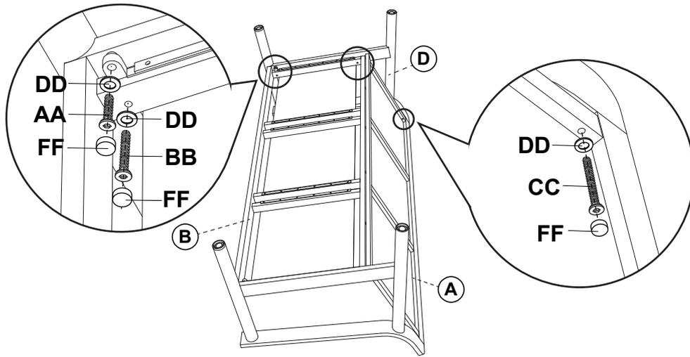
Attach the left chair leg (D) to the back (A) and seat (B) panel with bolts and washers, using allen key to tighten all the bolts.
