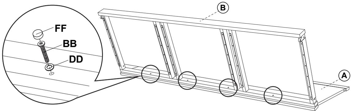
Attach the back panel (A) to the seat panel (B) with bolts and washers.
