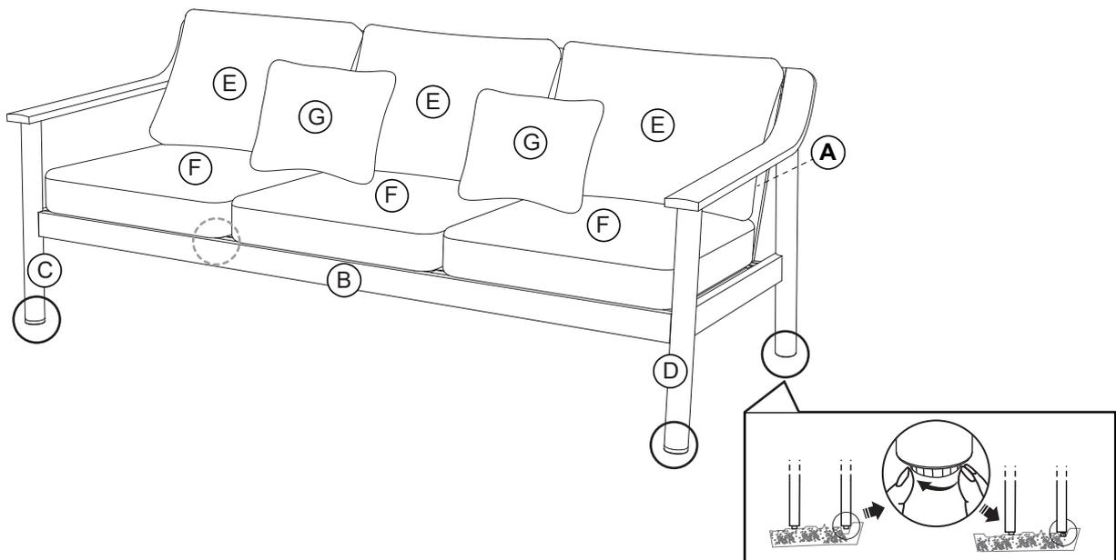
Attach the back cushion (E), seat cushion (F) and lumbar pillow (G) to the chair, adjust the foot leveler, assembly complete.
