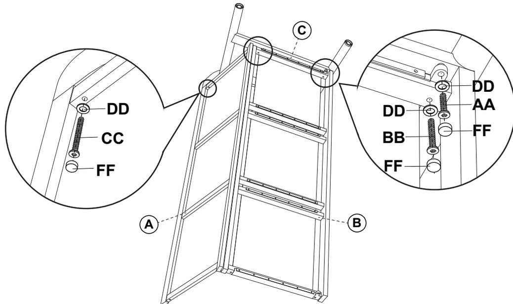
Attach the right chair leg (C) to the back (A) and seat (B) panel with bolts and washers.
