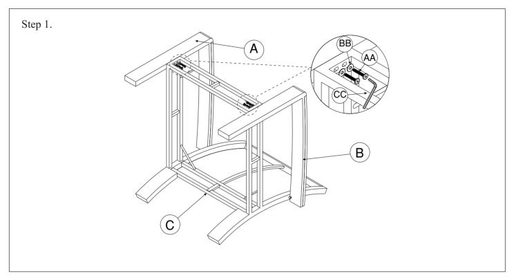
Assemble the side frame (A & B) into the seat frame (C) by bolt, flat washer. Using allen key to tighten all bolts
