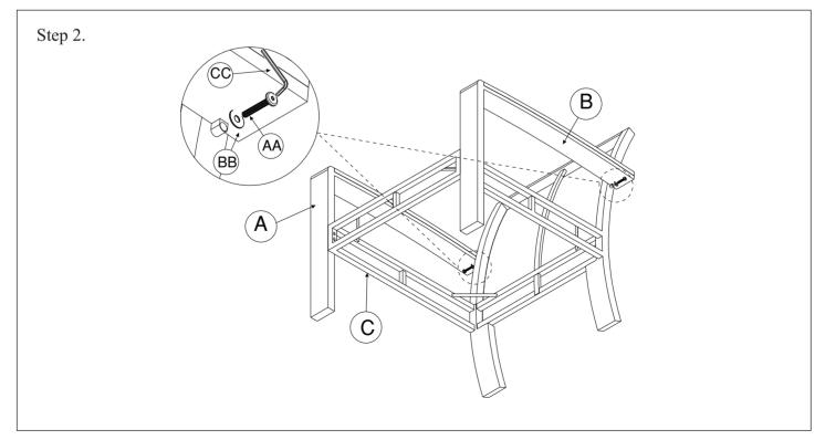
Assemble the side frame (A & B) into the seat frame (C) by bolt, flat washer. Using allen key to tighten all bolts
