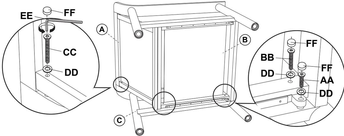
Attach the left chair leg (D) to the back (A) and seat (B) panel with bolts and washers, using allen key to tighten all the bolts.
