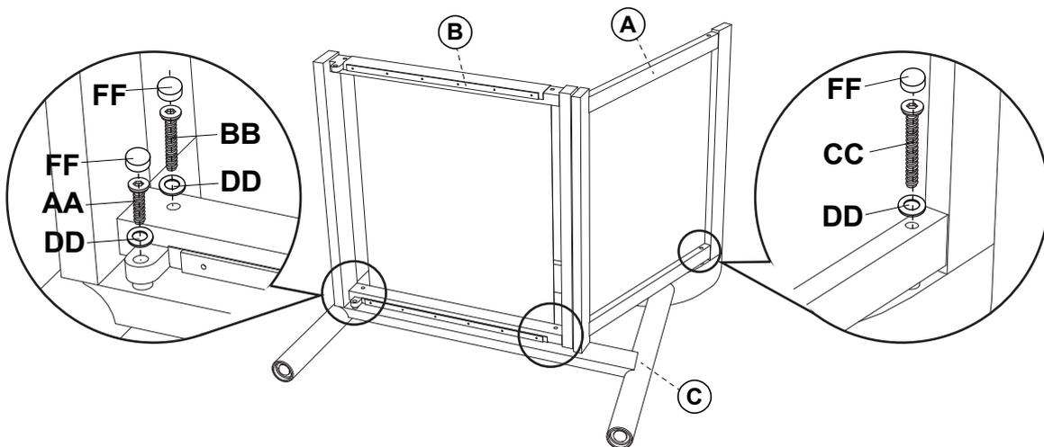
Attach the right chair leg (C) to the back (A) and seat (B) panel with bolts and washers.
