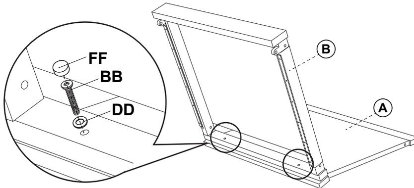
Attach the back panel (A) to the seat panel (B) with bolts and washers.
