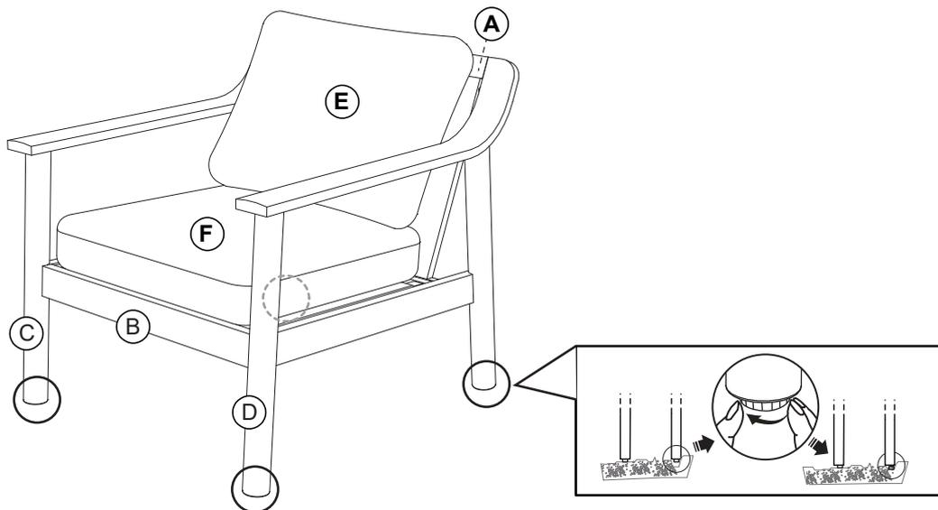
Attach the back (E) and seat (F) cushion to the chair, adjust the foot leveler, assembly complete.
