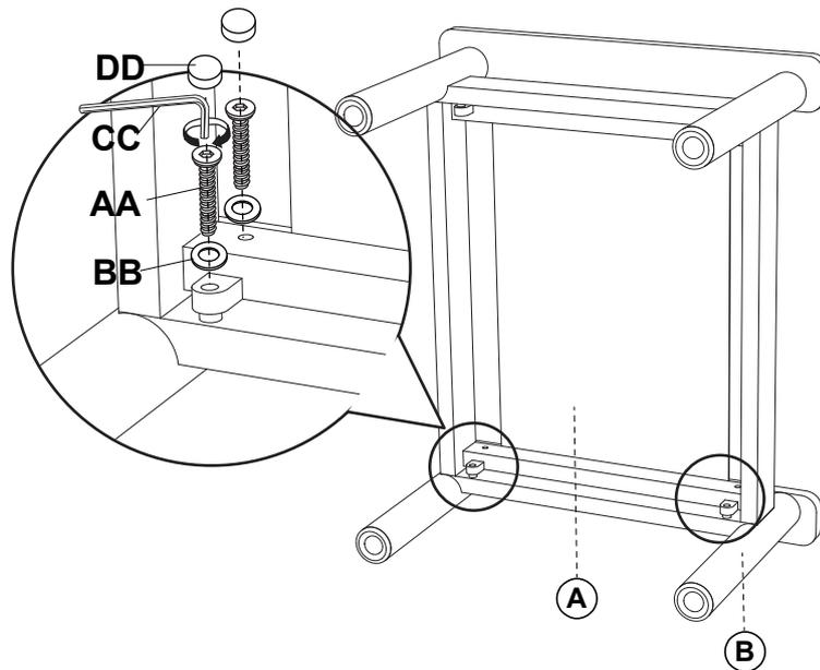
Attach the left leg (B) to the panel (A) with bolts and washers, using allen key to tighten all the bolts and then cover all caps.
