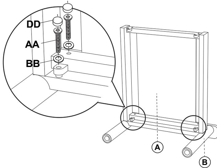
Attach the right leg (B) to the panel (A) with bolts and washers.
